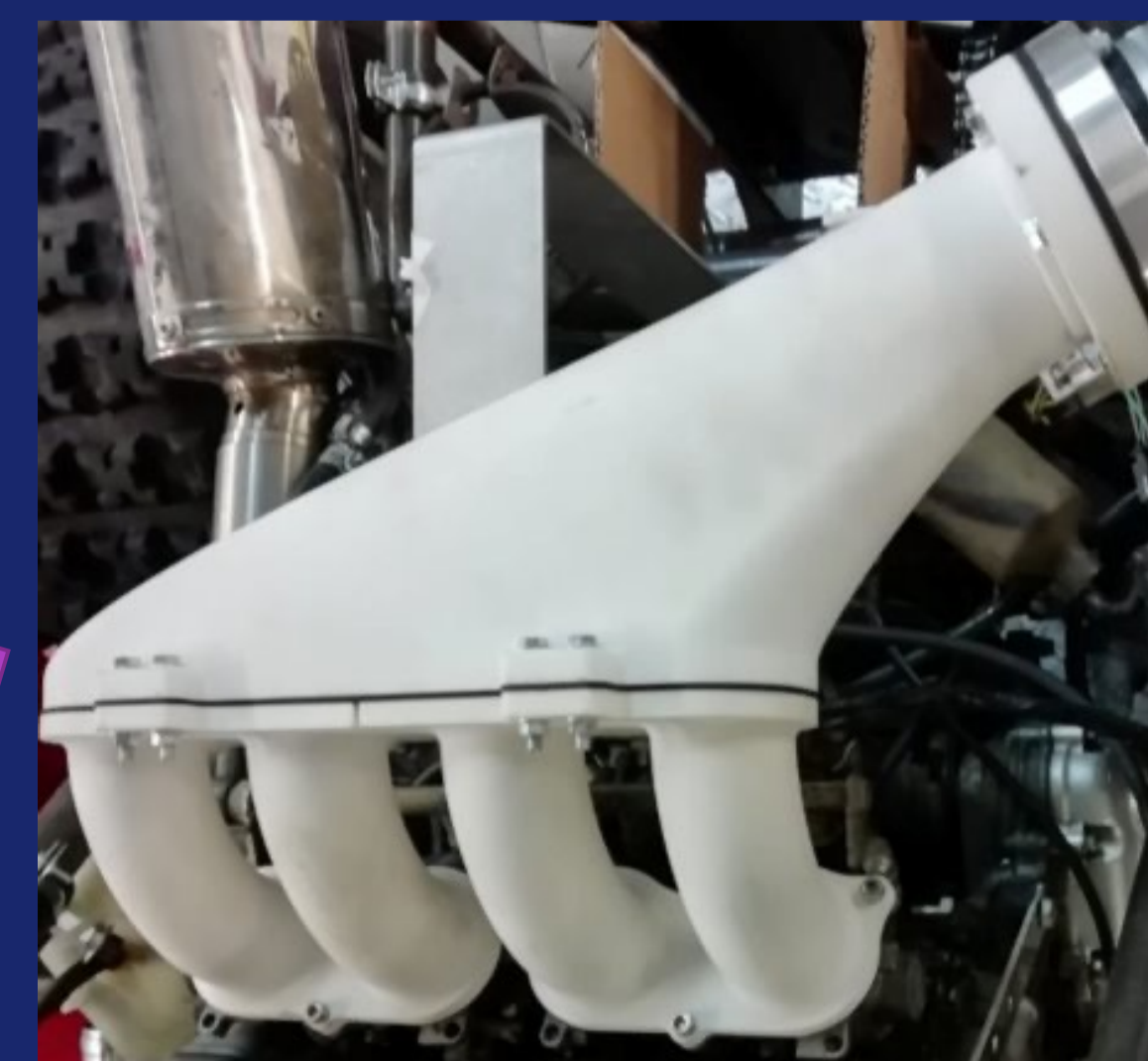
Figure 2. Final 3D printed intake manifold
