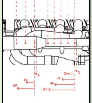
Impulse hammer test to find modal frequencies of least secure component.
