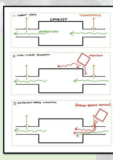
Catalyst **thermocouple tests** to investigate **light off time** and reduction strategies.
