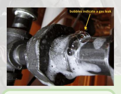
Soapy water gas leak test to assess joint manufacture quality.
