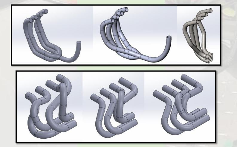
An initial design with piping routing through the bottom of the engine was developed.
