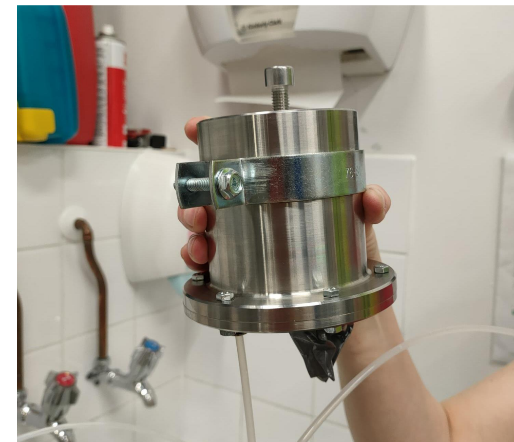
Assembled vessel with heating circuit removed
