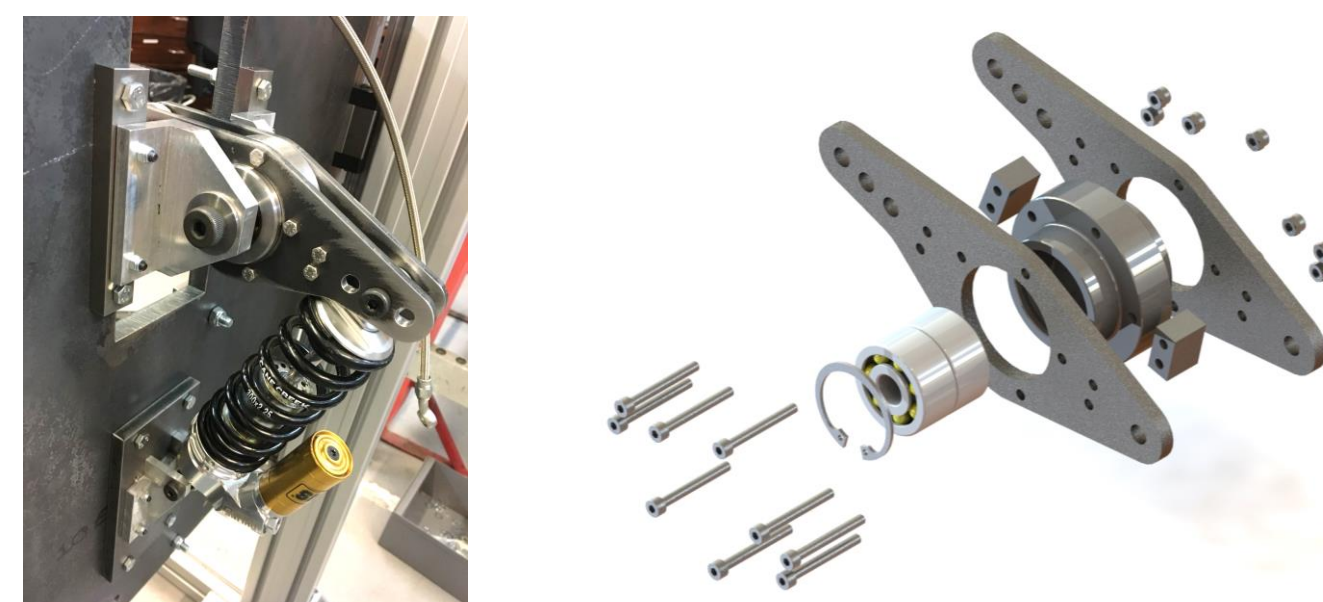
Figure 4: Render and photo of the rocker subassembly
