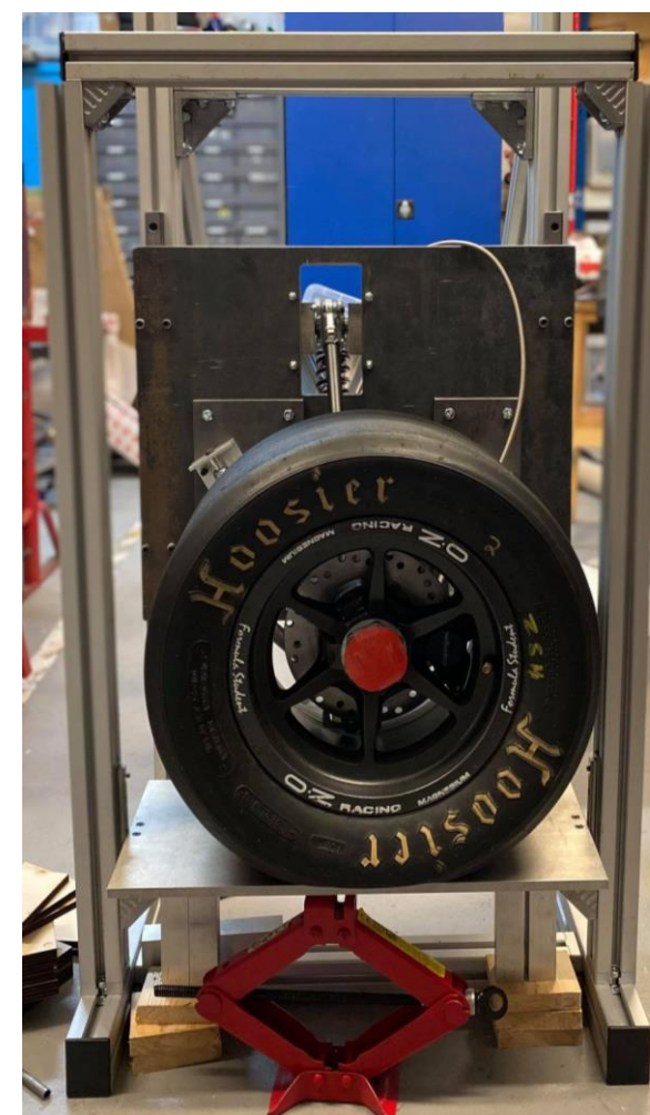
Figure 2: Quarter-car rig complete assembly
