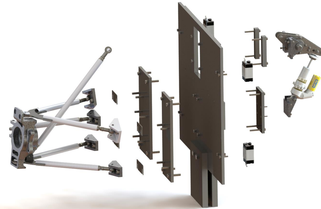
Figure 3: Mounting plate subassembly exploded view
