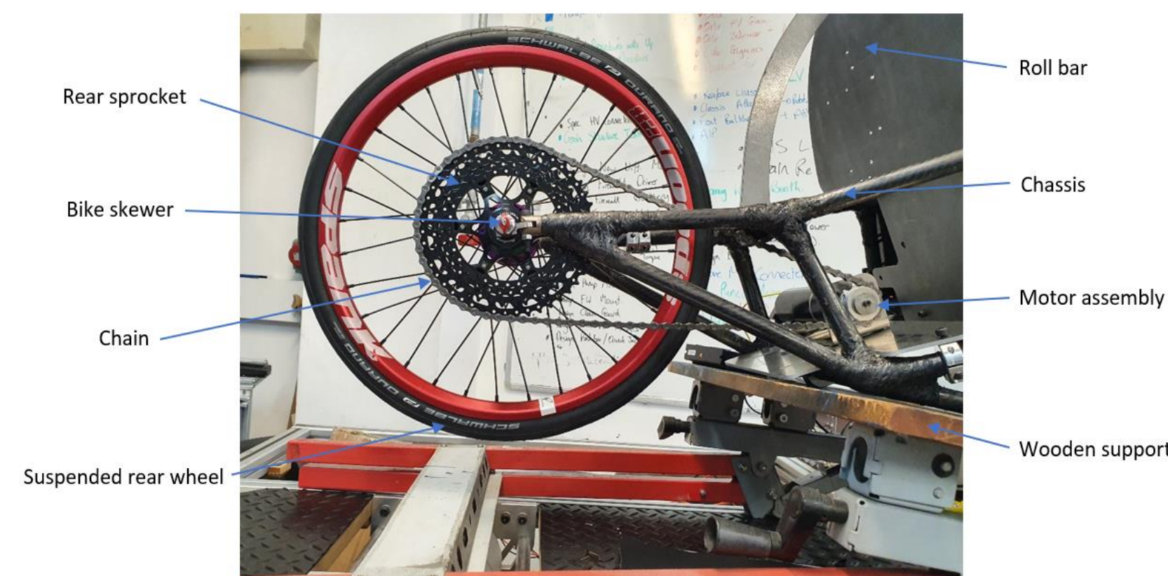
Labelled photograph of assembled powertrain
